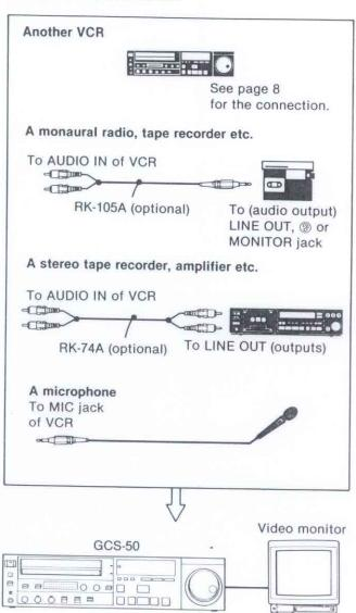
After the connection is made, set the switches on the VCR to the appropriate positions.
