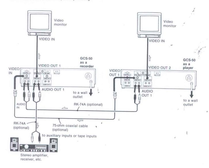
You can experience a more dynamic sound from tapes recorded in Beta hi-fi when the recorder is connected to a stereo system.
