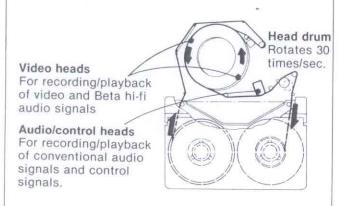
When the BETA HI-FI switch is set to ON, this recorder records audio signals both on the video track (Beta hi-fi recording) and on the conventional audio track (stereo) at the same time, so that these tapes can also be played back og any ordinary video cassette recorder without a Beta hi-fi system.
