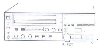
To eject the cassette, press the EJECT button. The CASSETTE IN indicator will go off.
