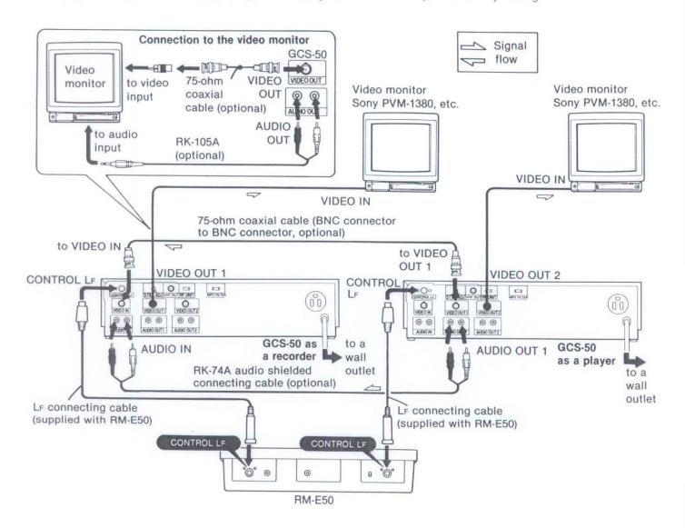
With the automatic editing controller, you will be able to preset the locations of the scenes you want to record (up to 64) in the controller, and with a press of a button, these scenes will be recorded automatically by the VCR in the preset order (assemble editing).
