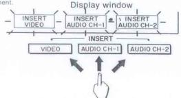
When these buttons are pressed, you will be able to monitor the sound and/or picture of the connected source.
