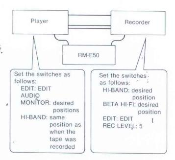
After making preparatory settings of the switches, start editing by operating the RM-E50. For details, read the instruction manual supplied with the RM-E50.
