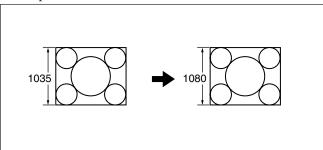
1035 ⇒ 1080 (PANEL): Convert the active scan lines from 1035 to 1080. Insert the 1035 lines into 1080 lines, then compress horizontally.
