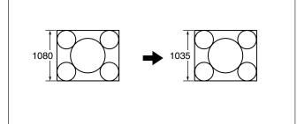
1080 ⇒ 1035 (CROP): Convert the active scan lines from 1080 to 1035. Crop the top, bottom, left, and right, then stretch the image horizontally.
