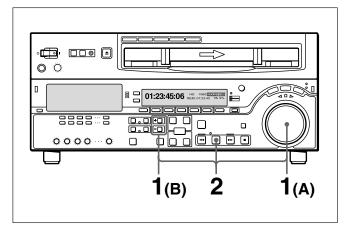
1 (A) Hold down the PLAY button, and turn the search dial in the desired direction to adjust the playback speed.
