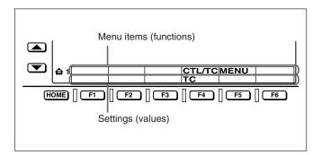
In the figure above, TC (time code) is selected as the setting for CTL/TC (time data selection), the menu item for button F4. This manual refers to this as "F4 (CTL/TC) in function menu HOME page is set to TC."
