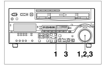
Press the SHUTTLE button or search dial so that the SHUTTLE button is lit.
