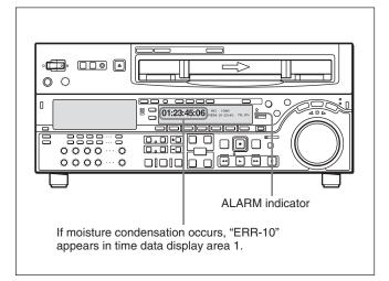
If this happens, the drum and capstan motors stop and the cassette is automatically ejected. Then, the drum starts to rotate again to dry its surface. In this state, the unit is not operable. When the moisture has evaporated, the error message disappears and the ALARM indicator goes off.
