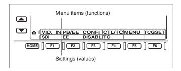
In the figure above, SDI (HD Serial Digital Interface signal) is selected as the setting for VID.IN (input video signal selection), the menu item for button F1. This manual refers to this as "F1 (VID.IN) in function menu HOME page is set to SDI."
