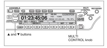
When the menu item number displayed in the menu display is flashing, you can change the menu item by turning the MULTI CONTROL knob.
