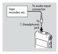
To record the sound of the IC recorder with other equipment, connect the  $\Omega$  (headphone) jack of the IC recorder to the audio input connector (minijack, stereo) of other equipment using an audio connecting cable\*.
