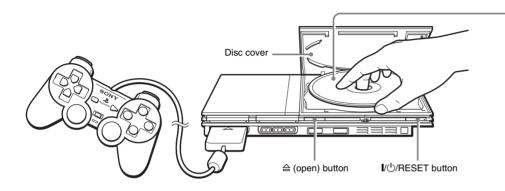
Place the disc in the console with the label side facing up.
