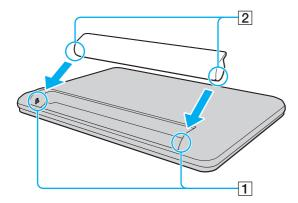
4 Push the battery pack down into the compartment until it clicks into place.
