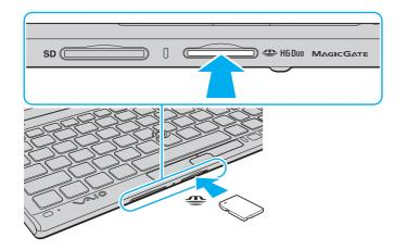
Before using "Memory Stick Micro" ("M2"), be sure to insert it into an "M2" Duo adaptor. If you insert the media directly into the "Memory Stick Duo" slot without the adaptor, you may not be able to remove it from the slot.
