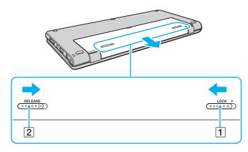
4 Hold the battery pack with your fingertips as illustrated below, lift it in the direction of the arrow, and then take it out of the battery compartment.
