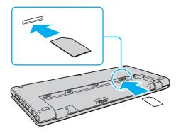
Do not touch the printed circuit on the SIM card. Be sure to hold your computer firmly before inserting or removing the card.
