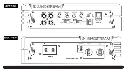
Class D Monoblock Amplifier Installation Wiring *LW1.1100D/LW1.1700D/LW1.2600D*
