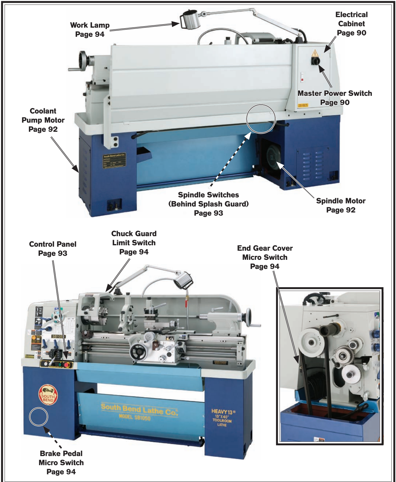
Figure 137. Component location index.
