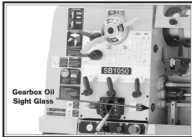
Figure 101. Location of quick-change gearbox oil sight glass.
