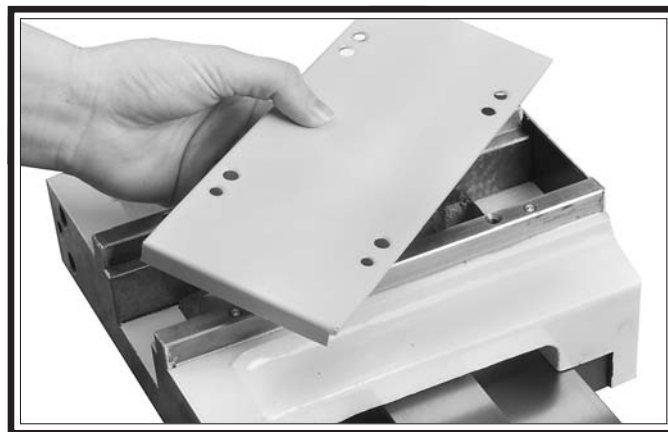
Figure 6. Top plate removal.
