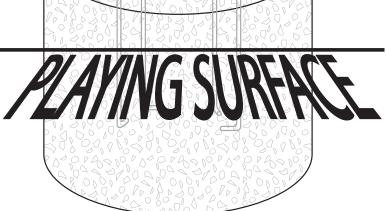
**IMPORTANT!:** WAIT A <u>MINIMUM</u> OF 72 HOURS BEFORE GOING ON TO NEXT STEP. CONCRETE <u>MUST</u> CURE. ALLOW ADDITIONAL TIME FOR COLD, WET OR HUMID WEATHER.
