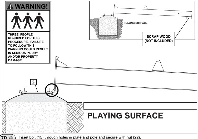
Insert bolt (15) through holes in plate and pole and secure with nut (22). 7B.♀
