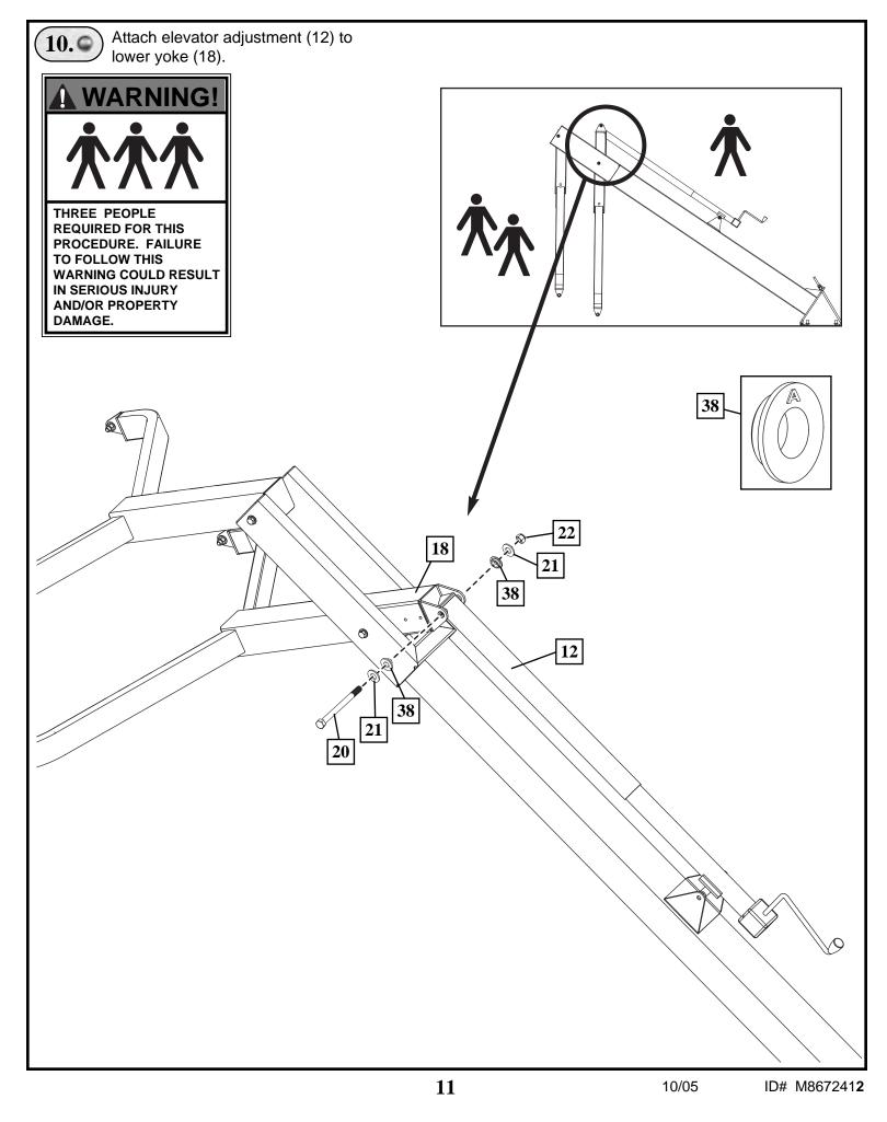
Attach elevator adjustment (12) to pole bracket.
