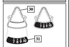
Attach height indicators to lower yoke in area shown by turning screws (29) into place with a Phillips head screwdriver. Apply name plate sticker (27) to lower yoke as shown.
