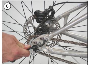
Tighten the two drive side bolts so that they're fixed, but not torqued to specification yet.
