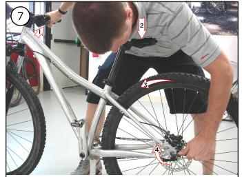
Apply downward force with body weight on the saddle and apply the rear brake, then roll the bike forward slightly. This will rotate the dropout as far forward as possible, so that the dropout won't be able to rotate under braking while riding.
