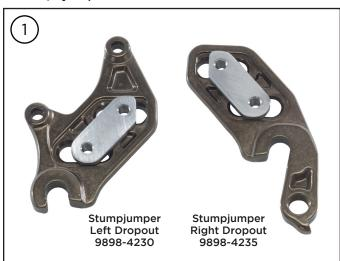
The bikes are equipped with one left and two right dropouts (with and without the derailleur hanger tab). After-Market dropouts are offered with the built-in derailleur hanger only and can be used with gears or as a single-speed dropout.
