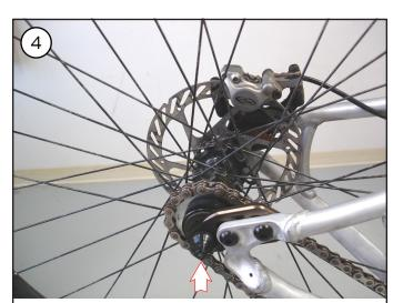
Install the rear wheel in the loose dropouts. Tightening the quick-release will self-align the wheel and dropouts.
