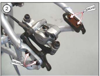
Install the left and right dropouts. The threaded steel backing plates are side-specific and must match the correct side dropouts.
