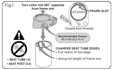
WARNING! Do not grease the seat tube surface that contacts the seat post. Grease reduces the friction that is critical to proper seat post grip. Remove any grease from the surfaces of the seat tube and seat post.
