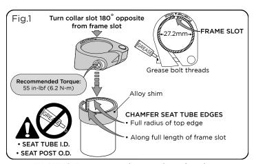
WARNING! Do not grease the seat tube surface that contacts the seat post. Grease reduces the friction that is critical to proper seat post grip. Remove any grease from the surfaces of the seat tube and seat post.
