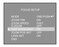
→ZOOM POS INIT: Moves to the controlled ZOOM position when the power t urned on and is a function of the initial ZOOM position control
