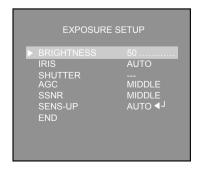
→IRIS: Set 'IRIS' to 'AUTO' or 'MANUAL'. Position the indicator over 'IRIS' us ing the UP or DOWN button and then select the desired iris mode usi ng the LEFT or RIGHT button.
