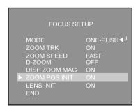
→LENS INIT: Use this feature to initialize the lens. Position the indicator over L ENS INIT. Using the UP or Down button. Press the SET button to confirm.
