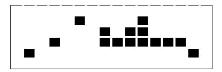
Use the Direction keys to move the cursor and press ENTER to select or de-select a grid. Press MODE to select all of the grids for detection; press MODE again to de-select all of the grids.
