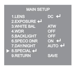
2. Select a desired mode using the Function Setup switch.
