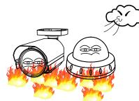
Only use the camera under conditions where temperatures are between -10°C and +50°C. Be especially careful to provide ventilation when operating under high temperatures. Do not install the camera under unstable lighting conditions.
