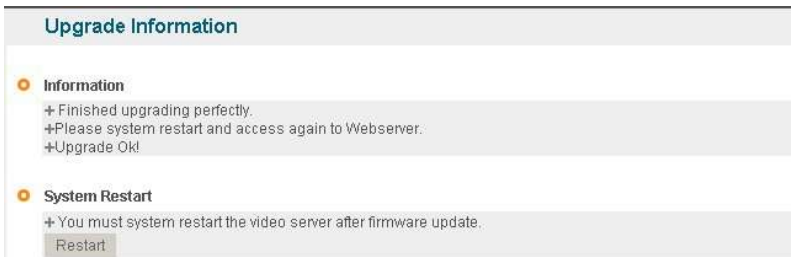
Fig. 4–25 Completion of Upgrade
