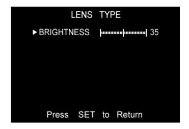
When DC LENS selected, press SET button to control the BRIGHTNESS.
