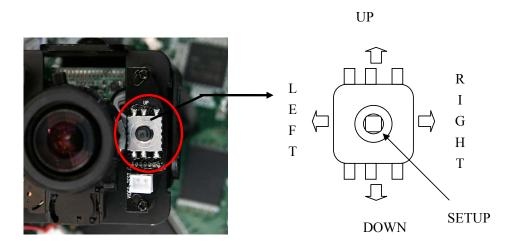
When you control by the five keys on the NVR Software GUI refer to the following
