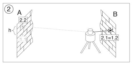
If the unit is within its working accuracy limits  $(\pm 20^\circ)$  the maximum difference from true level at 20 m (65 ft.) + 20 m (65 ft.) = 40 m (130 ft.) is 4 mm (3/16 inch).
