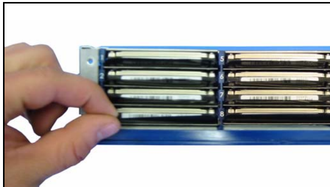
Figure 3-20 Pulling out the failed disk drive.
