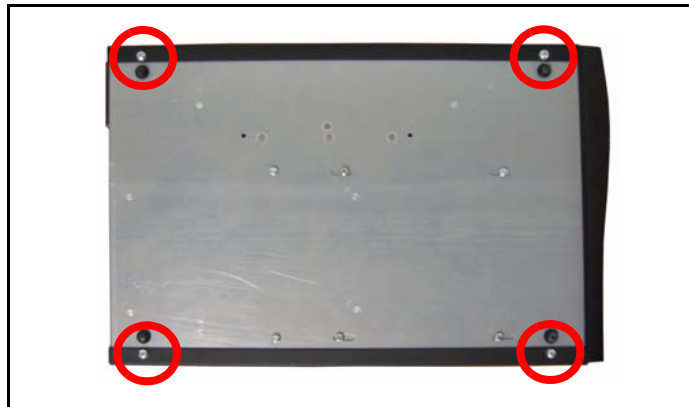
Figure 2-3 The four screws on the bottom of the unit.
