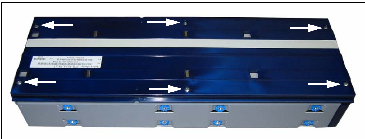
Figure 3-4 An Green RXT media pack with six screws to remove.
