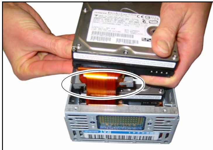
Figure 3-11 Sliding the bracket off the connector.
