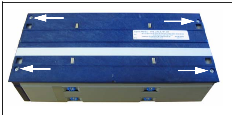
Figure 3-3 An Silver RXT media pack with four screws to remove.
