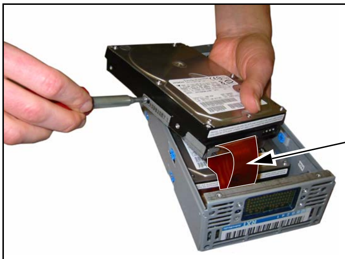
Figure 3-14 Securing the bracket to the disk drive.
