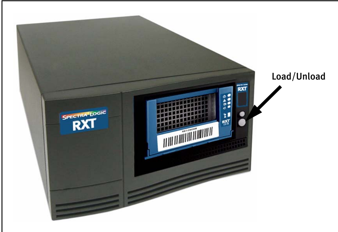
Figure 2-2 The Load/Unload button.
