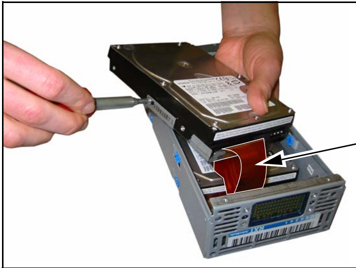
Figure 3-10 The bracket screw (Silver media shown).
