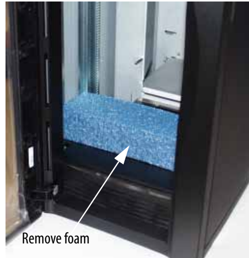
Figure 2-3 Remove the foam that protects the robotic picker from moving while shipping.
