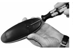
To remove the battery cover, use a normal screw driver. Insert it into the small crack behind the blind cover and break to open the handset.
