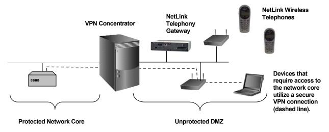
Deploying NetLink Wireless Telephones with a VPN
