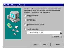
Select the CD that was delivered with the board as installation source. The driver files are located on CD in the directory
