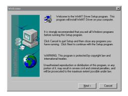
Under Windows NT the Spectrum driver must be installed manually. The driver is found on CD in the directory \Install\WinNTDrv. Please start the "Setup.exe" program. The installation is performed totally automatically, simply click on the "Next" button. After installtion the system must be rebooted once (see picture on the right side). The driver is install to support one PCI/PXI or CompactPCI
