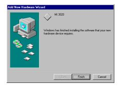
The drivers can be used directly after installation. It is not necessary to restart the system. The installed drivers are linked in the device manager. Below you'll see how to examine the driver version and how to update the driver with a newer version.
