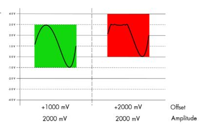
To avoid heavily distorted output signals please make sure to keep the signals in a range of ±3000 mV.
