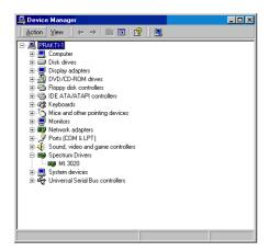
If you want to check which driver version is installed in the system this can be easily done in the device manager. Therefore please start the device manager from the control panel and show the properties of the installed driver.
