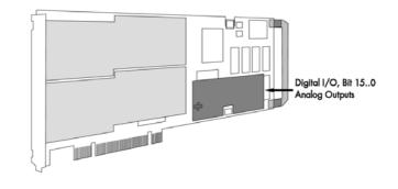
connector. The figure shows the position of this connector on the bottom side of the extra I/O piggy-back module. The shown option is mounted exemplarily on a board with two modules. Of course you can also combine this option as well with a board that is equipped with only one module
