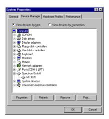
If you want to check which driver version is installed in the system this can be easily done in the device manager. Therefore please start the device manager from the control panel and show the properties of the installed driver.
