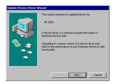
A new driver version is directly installed from the device manager. Therefore please open the properties page of the driver as shown in the section before. As next step click on the update driver button and follow the steps of the driver installation in a similar way to the previous board and driver installation.
