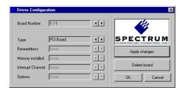
The Windows NT driver must be configured by the Driver Configuration utility to support more than one board. The Driver Configuration utility is automatically installed with the driver. The Utility can be found in the start menu as "DrvConfig".
