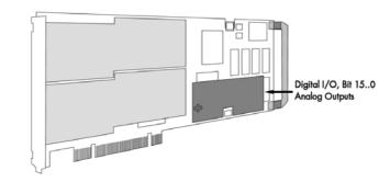
ket, but are available on an internal connector. The figure shows the position of this connector on the bottom side of the extra I/O piggy-back module.
