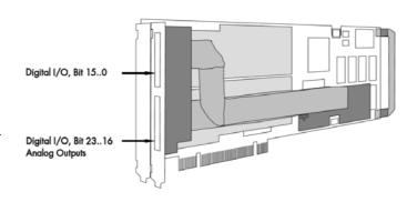
The additional inputs and outputs are mounted on an extra bracket.
