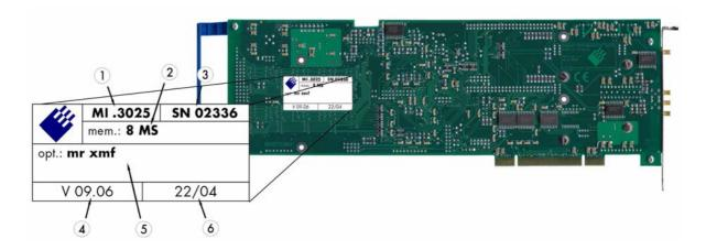
The Spectrum type plate, which consists of the following components, can be found on all of our boards.
