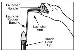
IMPORTANT: Hold the Launcher Handle as shown. Your thumb should be on the side of the Launcher where the Launcher Arm is attached.
