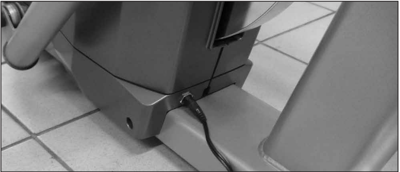
POWER CONNECTOR - Middle of unit
