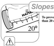
To prevent engine damage do not use the mower on slopes greater than  $20\ degrees$ .
