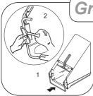
(1) Insert metal frame into grassbag fabric and (2) Clip into position.
