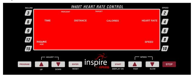
Note: Refer to upper drawing showing console display layout. IN400T display is shown, IN300T is similar. You have two option control choices for speed and incline. The right hand handle bar has a remote speed switch offering the same function as the display control keys. The left hand handle bar remotely controls incline.
