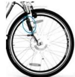
As the front wheel contains the hub motor, there are additional steps in the case you require the entire wheel to be removed from the bike.
