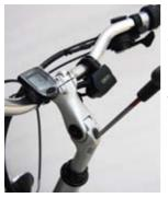
Handlebar / Stem / Headset Handlebar and stem comes pre-assembled. Loosen bolts on the stem and insert and turn the handle bar assembly until it is in right angles with the frame. Then tighten. Tightening torque 18 Nm
