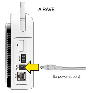
Insert one end of the power cord into the power supply. 5
