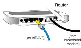
**3** Connect the other end to the WAN port located at the rear of the base station.
