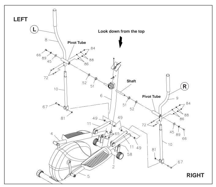
**STEP 8:** There is an "L" decal on the LEFT HANDLEBAR(8), and an "R" decal on the RIGHT HANDLEBAR (9). To assemble the RIGHT HANDLEBAR(9), place a SPACER(51) and a LARGE WASHER(M16)(52) on the right side of the SHAFT on the UPRIGHT(6). Slide the RIGHT HANDLEBAR(9) onto the SHAFT and secure with a LARGE WASHER(M8)(45), LOCK WASHER(M8)(89), and BUTTON HEAD BOLT (M8x1.25x20mm)(66). Repeat on the left side.
