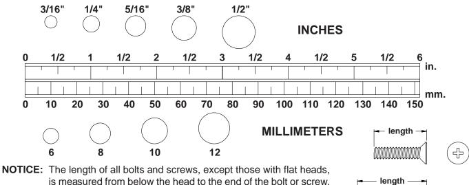
Flat head bolts and screws are measured from the top of the head to the end of the bolt or screw.
