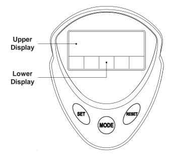
Stop pedaling for four seconds. Press the **MODE** button to select functions for preset target values. The meter will cycle through the functions as follows and allow you to set the function values.
