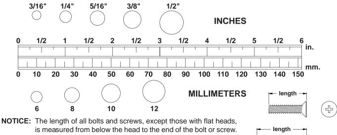
Flat head bolts and screws are measured from the top of the head to the end of the bolt or screw.
