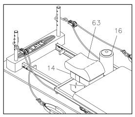
Make sure that both FOAM PADS(16) are in the carriage when using the HEADPAD(63) attached to the HEADREST(14).
