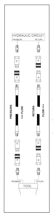
Figure 1. Typical Hose Connections
