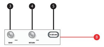
**3. Send Level:** Controls the output level (send volume) of the FX Loop when a channel's effects send (#40) is activated.
