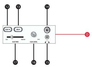
**12.** Cue FX: Sends the effected signal from the FX Loop to the Headphone Cue for monitoring (see Section-B.) This allows DJs to hear what the FX Loop sounds like, before sending it to the Master Outputs.
