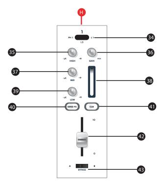
**34. Input selector switch:** Selects phono or line input for the corresponding channel. This is a three way switch allowing input from only one device at a time (Phono or either of two Line level inputs (for connections in rear panel of mixer, see Sections N-R.)
