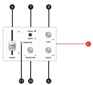
**6. Master Level:** Controls the overall output level of the audio signal sent through the Master connectors (see Output Connections.)
