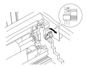
□ Move the adjustment lever on the right side of the platen to one of its four settings. The adjustment lever position that is nearest to the back of the printer is Position 1 (minimum gap), while the position at the opposite extreme is Position 4 (maximum gap). Position 2, which is marked with a dot, is most suitable for single-sheet paper.
