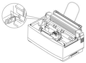
□ Lower the automatic feeder all the way down. When you do, it should naturally slip into place, with the part that holds the paper angled slightly towards the back of the printer.
