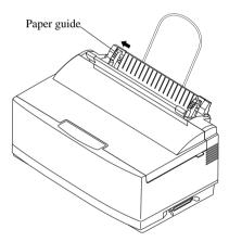
□ Pick up the stack of paper with both hands, and fan through the paper with your thumb. This prevents paper from sticking together when it is fed by the automatic feeder.
