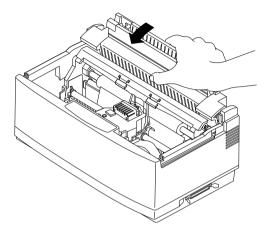
□ Lift the automatic sheet feeder straight up.
