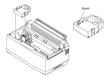
□ If you have a color printer model, be sure to carefully position the ribbon between the print head and the print head shield as shown in the illustration.
