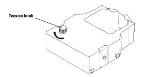
• Gently lower the cartridge into the cartridge holder. Make sure that the spindle on the cartridge holder fits into the socket on the base of the cartridge.
