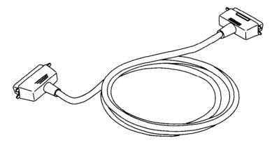
The parallel cable has a 25-pin "D-type" plug at one end, and a 36-pin Centronics connector at the other. Plug the 25-pin plug into the parallel socket on your computer. This will probably be labelled **Printer**, **Parallel**, **PRN**, **LPT1** or something similar.
