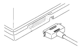
Secure the connector with the clips as shown.
