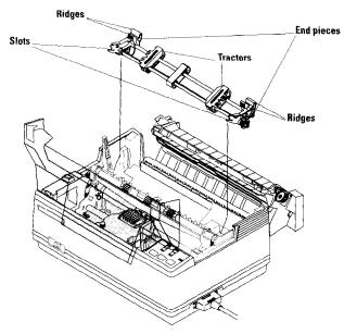
• Hook the slots in the end pieces over the shaft just behind and above the platen roller.
