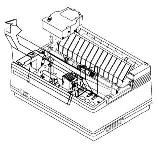
• Carefully position the ribbon between the print head and the print head shield as shown.
