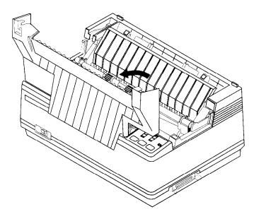
Note: If you wish, you can remove the front cover completely. However, we strongly recommend that you put it back on the printer again as soon as you have installed the ribbon cartridge. This cover prevents objects that may damage the printer from getting inside it, and also reduces printing noise.
