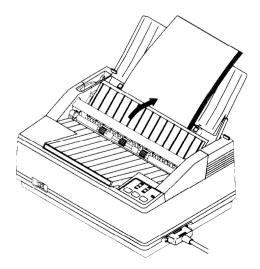
• Push the paper delivery selector up and back. Printed pages will now be delivered in a stack, face down. When you turn the stack of printed pages right-side up, the sheets will be in the order in which they were printed.
