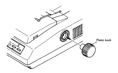
The platen knob should be removed from the accessory box inside the shipping carton. Mount the platen knob on the shaft on the right-hand side of the printer. Turn the knob on the shaft before pushing the knob fully into position.
