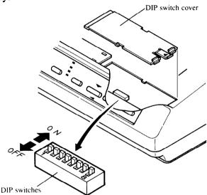
Access the switches by removing the top cover, and then sliding the black switch cover to the left and then pulling up, using the tab at the right, as shown in the illustration above.
