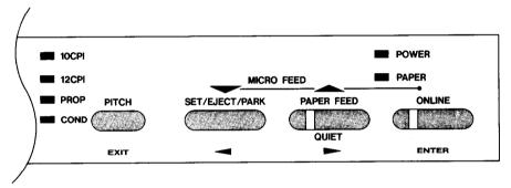
The principle involved is that the printer will print a list of options on one line. You use the Setelecters and Paper FEED buttons to move the print head so that it is below the option you want to choose.
