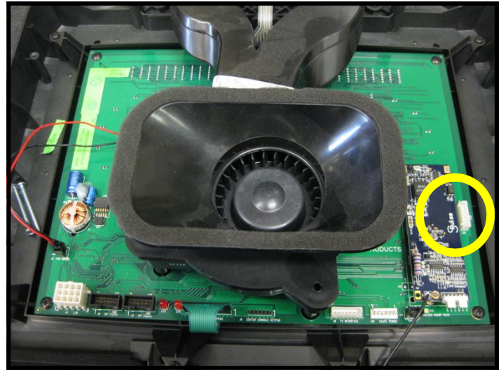
Step 22. Connect the seven-pin interface cable from the console to J14 connector on the display board.
