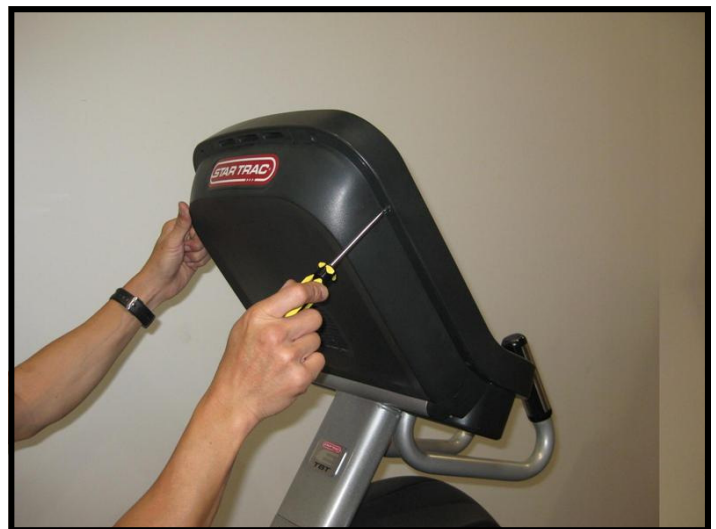
Step 20. Using a Phillips head screw driver, secure the front display to the back with (8) M4 x 0.7 x 19mm long Phillips head screws.
