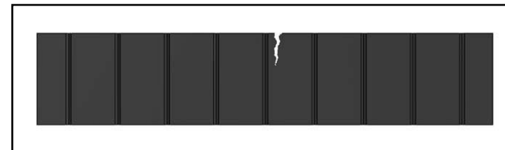
■ Torn or cracked belt
