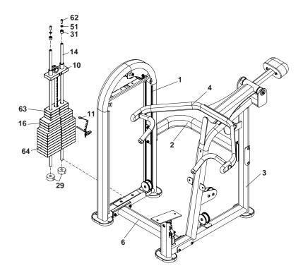
Install the top plate (10) on the weight stack guide posts (14), inserting the top plate shaft through the holes in the weights. Insert the selector pin (11) through one weight until it engages the top plate shaft.
