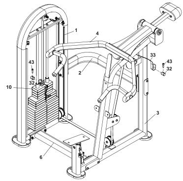
Insert one end of the weight belt (33) through the slot in the top plate belt clamp until approximately one inch of the free end of the belt protrudes from the slot in the opposite side of the clamp.
