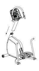
(c) Thread in (4) M6 x 16 Flat Head Screws in the front and back of the neck where the two pieces came together. Us a 5/32 hex key to tighten the screws to 60 lb-in (6.7 N-m) of torque.
