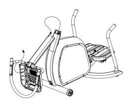
(b) Keep hold of the cables and rotate the display up. Now slide the neck over the two mount in the lower neck, take special care not to pinch the cables or your finger when the two pieces come together.
