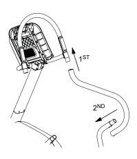
(e) Use a 5/32" Hex Key and thread into the handrail (2)  $1/4-28 \times 3/8$ " Button Head Screws into the upper handrail. Then tighten each screw to 110 lb-in (12.4 N-m) of torque.
