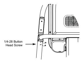
(f) Use a 5/32" Hex Key and thread into the handrail (2)  $1/4-28 \times 3/8$ " Button Head Screws into the lower handrail. Then tighten each screw to 110 lb-in (12.4 N-m) of torque.
