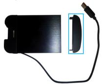
Instruction Manual Statechcom Download from Www.Somanuals.com. All Manuals Search And ซีซีฟีฟิเซิส์. 3. Connect the the 2.5" SATA Hard Drive by sliding it into the enclosure connector first.
